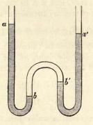
The columns a b, a' b', of mercury are each exposed to the pressure of the atmosphere at their upper ends, and at their lower ends to the pressure of the air in b b'. Hence, if the differences of level of the surfaces at a and b, and at a' and b', be measured with a cathetometer, the mercury in each tube has a density inversely as the corresponding measured number.
